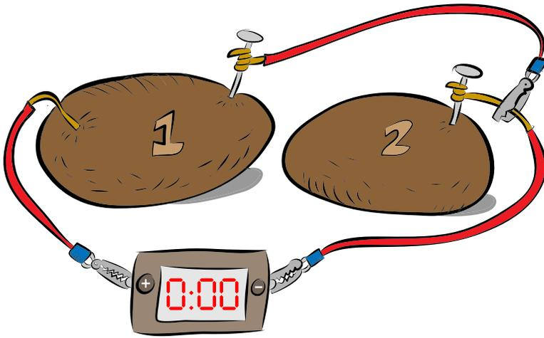
**B**elieve it or not, an ordinary potato can also be a battery! The potato you eat for supper has enough electrochemical energy to power a small watch! Small amounts of acid and salt in the potato make an excellent conductor. Let's set up an experiment and see if it works!
